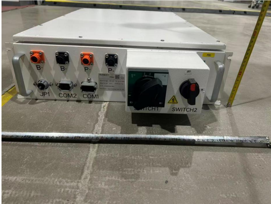
Picture 17 High voltage box/PDU with DC/DC module (Front view)
