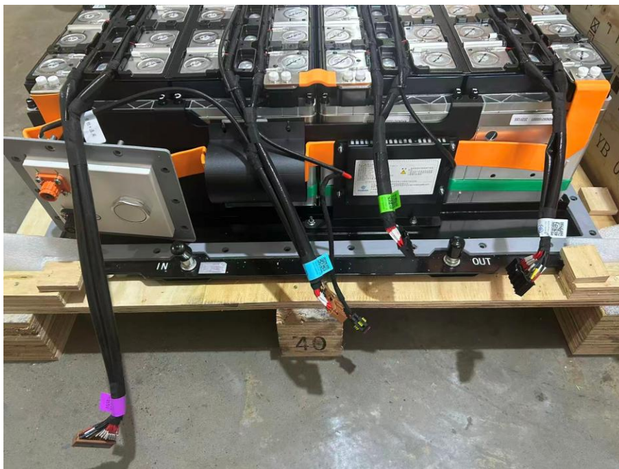
Picture 16 Battery pack (Inside view 2)
