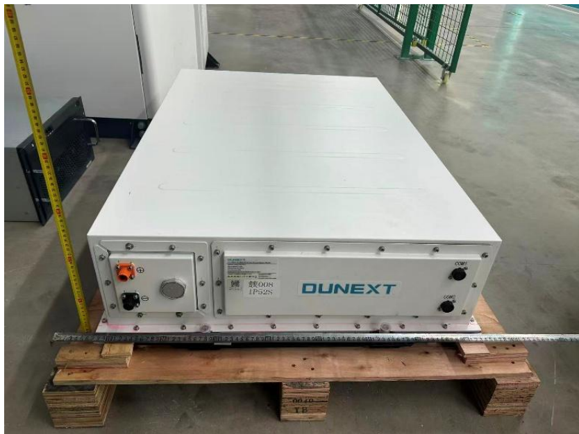
Picture 12 Battery pack (Top and front view)
