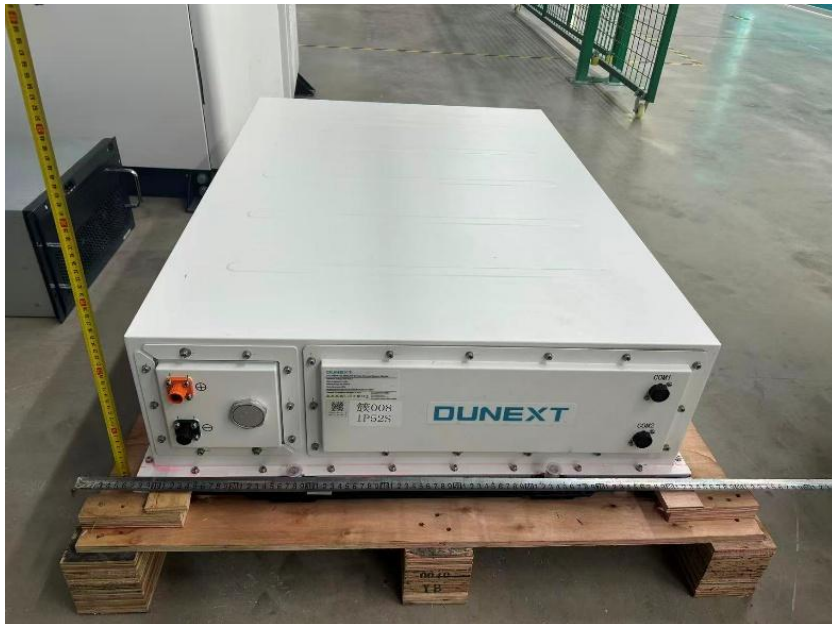
Picture 12 Battery pack (Top and front view)
