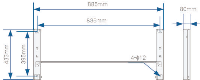
Figure 6-1 Dimensions of Mounting Bracket
