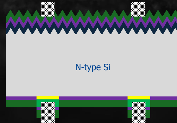
TOPCon-Poly Tech cell structure
