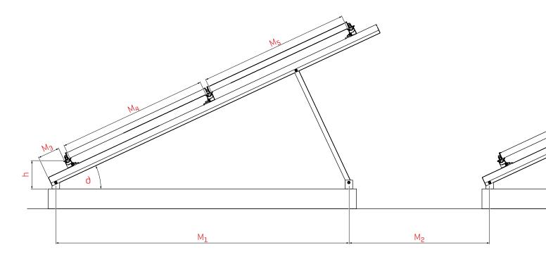
h = Space between ballast/ground and module under edge
