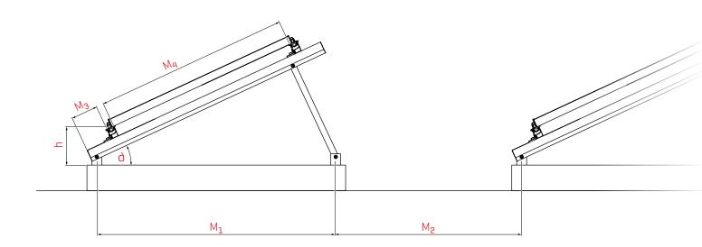
h = Space between ballast/ground and module under edge
