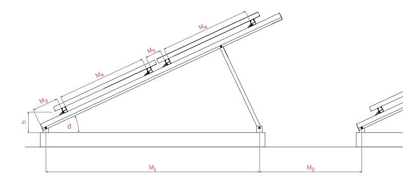
h = Space between ballast/ground and module under edge
