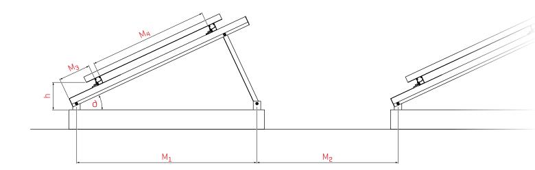
h = Space between ballast/ground and module under edge
