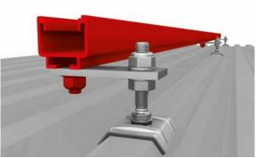
Ensure correct position of T-bolt. After inserting into the lower chamber of the rail, the T-bolt is turned 90 degrees counterclockwise. Lock the projected K2 module carrier rail Solid on the adapter plate with an M10 T-bolt and tighten.
