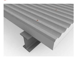
Measure the screw distances according to statics or K2 Base. Check position of purlins and pre-drill through the profile sheets into the purlins.
