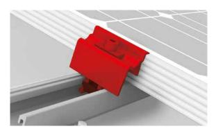
Fix the module in place at the end of a row with universal module end clamp OneEnd. Klick the Stance in the notches. Alternatively use the standard end clamp. Insert the MK2 nut into the mounting rail and turn clockwise by 90°. Place clamps on the module frames and fix them. Never mount module end clamps directly on the rail joint or end of the rail! (Spacing: min. 50 mm from edge of module frame). Pay attention to the mounting instructions by module manufacturer!
