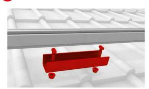
Lay Mounting Rail on joint with rail connector and connect with T bolts and self-locking nuts. The rail joint may not be in the range of the roof fastener. Tightening torque 16 Nm.
