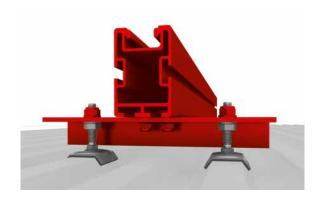
The K2 Bridge is mounted on two solar fasteners instead of the adapter plate in order to achieve greater span widths. Depending on type, the rail is fixed to the Bridge with one or two M10x30 T-bolts.
