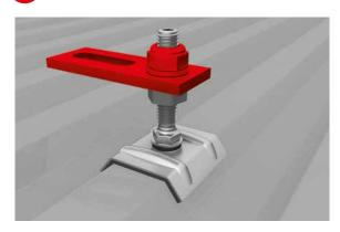
Place adapter plate, adjust and mount additional washer with locking nut.
