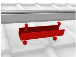
Lay Mounting Rail on joint with rail connector and connect with T bolts and self-locking nuts. The rail joint may not be in the range of the roof fastener. Tightening torque 35 Nm.
