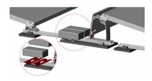
Depending on ballast size, position each SpeedPorter with the appropriate distance and insert the ballast. See page 15.
