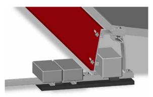
Use a ballast with the Dome \$1000 2.0 where necessary. See page (see page 15) and fix module cable in place.
