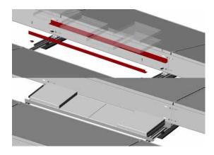
Fix Porters (L-brackets) in place on the parallel SpeedRails with MK2 slot nuts and countersunk screws.
