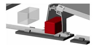
For ballast of up to 5 kg, one or two individual weight bricks can be placed in the cavity of the \$1000 2.0. See page 15.
