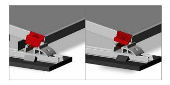
Fix the module in place at the end of a row with universal module end clamp OneEnd. Klick the Stance in the notches. Place clamps on the module frames and fix them.
