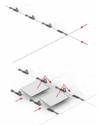
Pre-assemble all Dome components on the short rails accordingly and install on the roof according to the following scheme:
