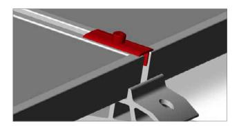
Between every two modules, use two XS middle clamp sets. Insert clamp sets in the S1000 and SD 2.0 notches and rotate 90°. Place the clamps onto the module frame and fix them in place.
