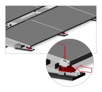
The modules are laid horizontally, in the centre of two Dome D1000s. The specially affixed bars serve as the stop. Thereafter, the module is positioned on two Dome SDs. The only loosely fastened Dome SD together with the protection mat SD  $160 \times 180 \times 18$  mm are pushed towards and against the module and then fastened. Before fastening ensure that the WINGS of the protection mat are under the Dome SD and the rails at the array edges do not protrude. Tightening torque: 16 Nm.
