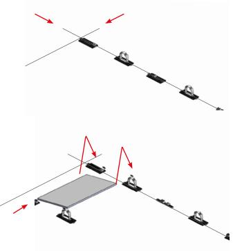
Pre-assemble all Dome components on the short rails accordingly and install on the roof according to the following scheme:
