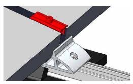
Between every two modules, use two XS middle clamp sets. Insert clamp sets in the D1000 and SD 2.0 notches and rotate 90°. Place the clamps onto the module frame and fix them in place.
