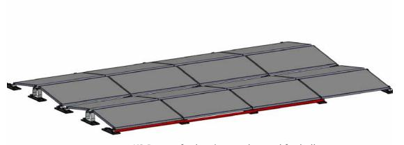
K2 Porters for bracing can be used for ballast reduction in the corner areas. According to the technical design, these must always be positioned on the three outside modules.
