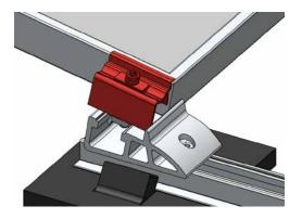
Fix the module in place at the end of a row with universal module end clamp OneEnd. Klick the Stance in the notches. Place clamps on the module frames and fix them.
