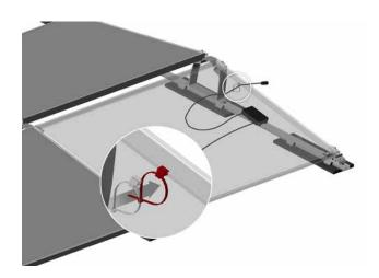
Bend the K2 Solar Cable Manager to a circle and plug it into the module frame backside. Then insert the cables through the cable tie.
