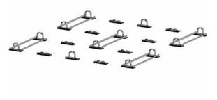
Mount the Porters within a module block according to the drawing in an offset fashion, and distribute the ballast evenly.
