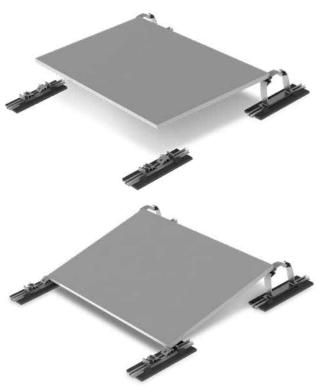
Fasten module clamps sets to the end of the row. Attach the D1000 and SD 2.0 with MK2 slot nuts and clamps and rotate 90  $^{\circ}$ . Fasten clamps to the module frame with an allen bolt.
