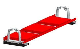
Fix Porters (L-brackets) in place on the parallel SpeedRails with MK 2 slot nuts and countersunk screws.
