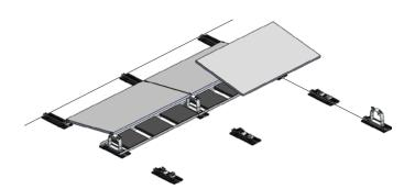
Mount modules on opposite sides (Ensure that the clamps are securely seated).
