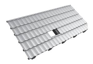
The rafters, where the roof hooks will be fixed to, have to be uncovered. In case of timber boarding or sarking boards instead of battens the exact position of the rafter has to be determined to ensure proper fixing of the roof hook.
