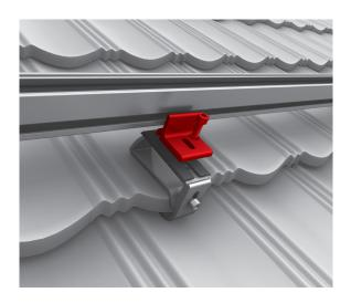
The mounting rail is mounted on the roof hook with the help of of the K2 Climber and the Allen bolt with underhead serration. Tightening torque 16 Nm.
