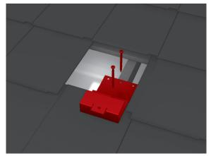
The roof fastener must be mounted with a minimum of two stainless steel timber screws on the wooden rafters (at least one screw per row of holes). The large surface of the roof fastener must be placed flush on the surface of the underlying large interlocking plain tiles. The roof fastener may not be mounted over a lateral overlapping of the concrete tiles.
