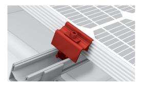
Fix the module in place at the end of a row with universal module end clamp OneEnd. Klick the Stance in the notches. Alternatively use the standard end clamp. Insert the MK2 nut into the mounting rail and turn clockwise by 90 °. Place clamps on the module frames and fix them. Never mount module end clamps directly on the rail joint or end of the rail! (Spacing: min. 50 mm from module end clamp). Pay attention to the mounting instructions by module manufacturer!
