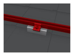
The Mounting Rail is mounted on to the roof fastener using K2 Climbers and K2 Bolts with serrated under head. Tightening torque 16 Nm.
