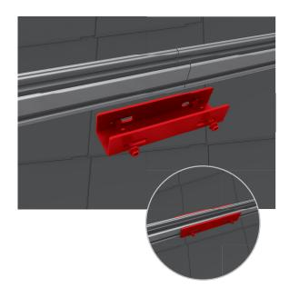
Lay Mounting Rail on joint with rail connector and connect with T bolts and self-locking nuts. The rail joint may not be in the range of the roof fastener. Tightening torque 16 Nm.
