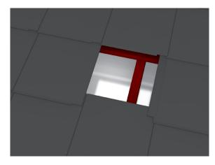
The rafters, on which the roof fasteners are to be mounted, must be exposed. The height of the roof fastener must be checked and adjusted if necessary.
