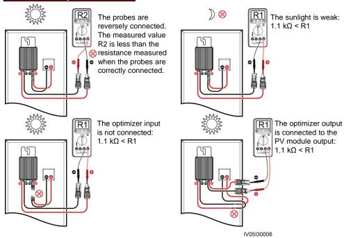
Check that the optimizer input is properly connected, and connect the output power cables to the optimizer. Measure the PV string resistance when the sunlight is sufficient.
