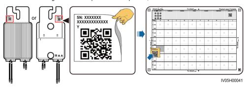
2. Install the optimizer based on the selected installation mode.
